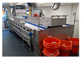
CU TCD is specialized in engineering, production and installation of catch processing equipment, intended for the processing of fresh fish onboard fishing vessels. Complete Catch Processing Systems, including conveyor and transport belts, (bubble-jet) washing machines, gutters, collection bins, grading and weighing solutions, cooling- and (slurry) ice machines.
